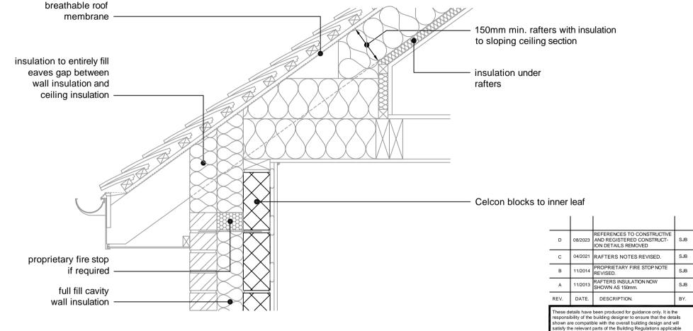
This junction detail has been assessed by H+H UK Ltd. for thermal performance based on various Celcon blocks and insulation combinations. Applicable Ψ-values and minimum temperature factors compatible with the latest Building Regulations can be found in our 'H+H Calculated Ψ-values' document, available to download from our website www.hhcelcon.co.uk.
